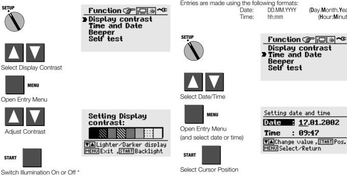
Background illumination is switched off automatically after approximately 2.5 minutes if none of the keys are activated during this time. Each time a key is activated, background illumination is extended for an additional 2.5 minutes.
