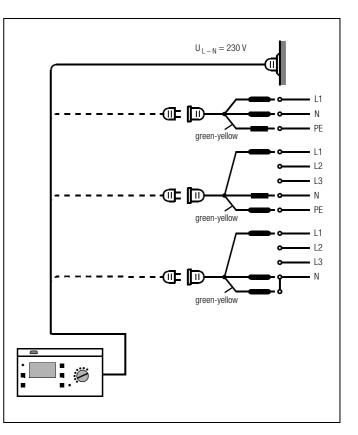
➡ Connect the test instrument to 230 V or 120 V mains power (depending on the country-specific design) with the included mains connector cable.
